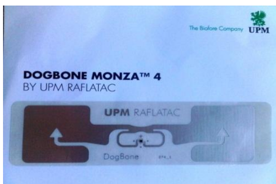
Fig.2: Real implementation of RFID tag (Courtesy of UPM RAFLATAC)
